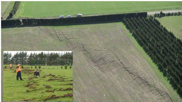
**Figure 2:** Surface rupture of the Greendale fault, close to Highfield Road, North Canterbury viewed from the air and ground (inset). At this point there was about 4 m horizontal movement and over 1 m vertical movement on the fault (Main photo: Russel Green, GEER; Inset: University of Canterbury).
